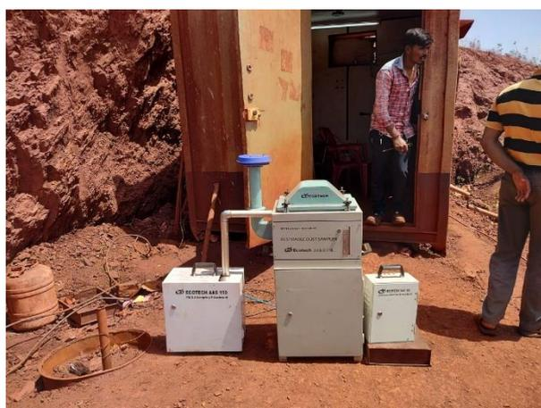
**Fig. 3: Dust sampling using a respirable dust sampler (Ecotech AAS 190) (PM10) and Particulate dust sampler (Ecotech AAS127) (PM2.5)**
